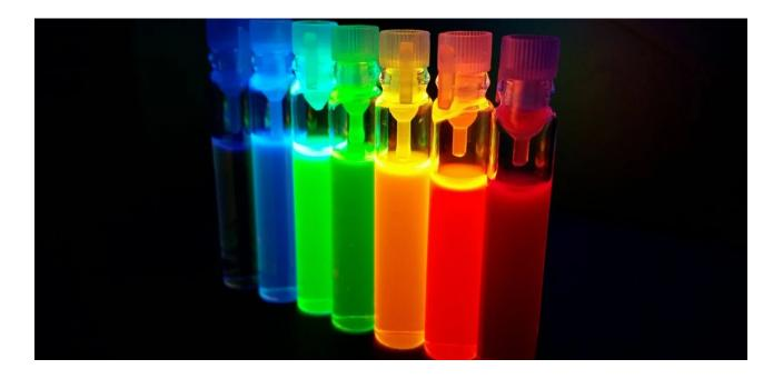
Glass tubes with quantum dots of perovskite nanocrystals, luminescing under ultraviolet radiation
